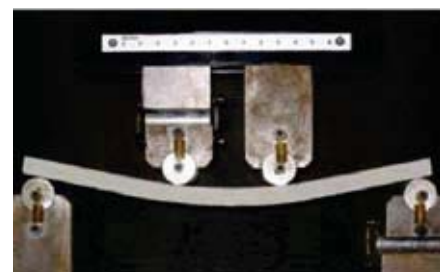
This image shows the unique properties of engineered cementitious composites in both their high ductility and ability to self-heal after fracture.
