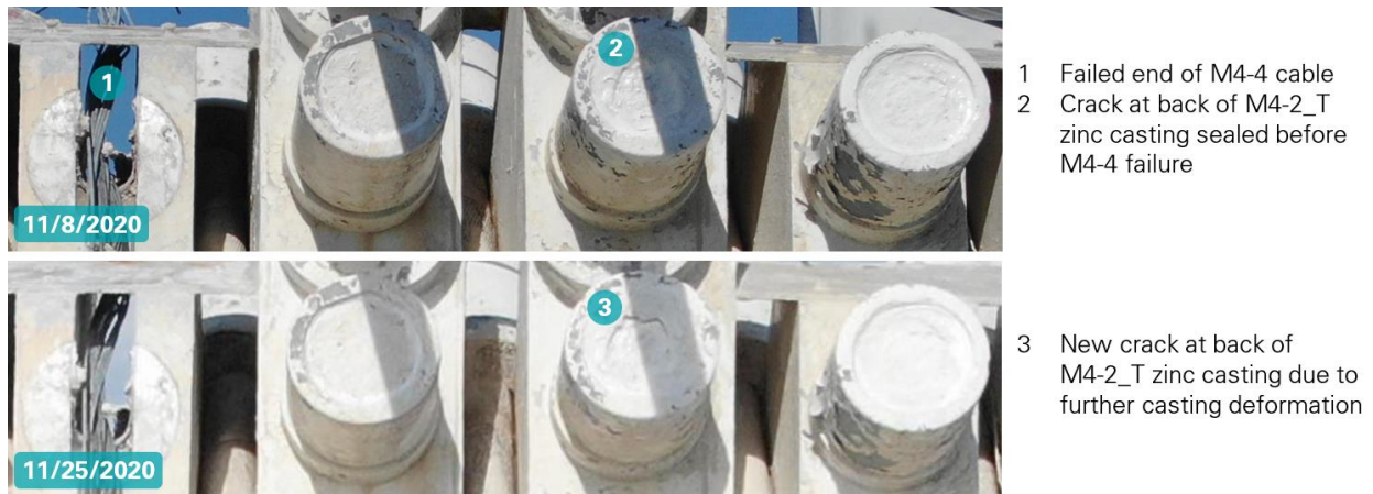
Figure 28: Evidence of socket casting core displacement after second cable failure (photos: NAIC Arecibo Observatory, a facility of the NSF).
