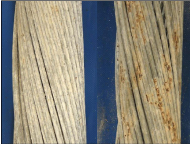
Figure 30: Oxidation of galvanizing zinc (left) and wire steel (right) in second wire layer of an original M4 cable (photos: Socotec).
