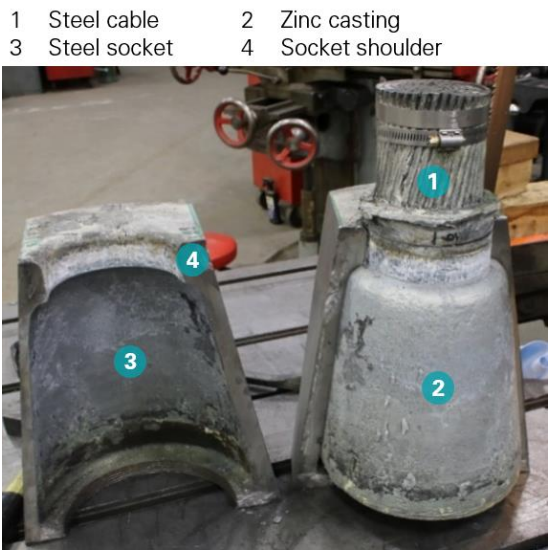
Figure 5: Zinc casting of auxiliary backstay socket B4N_G (photo: Socotec).
